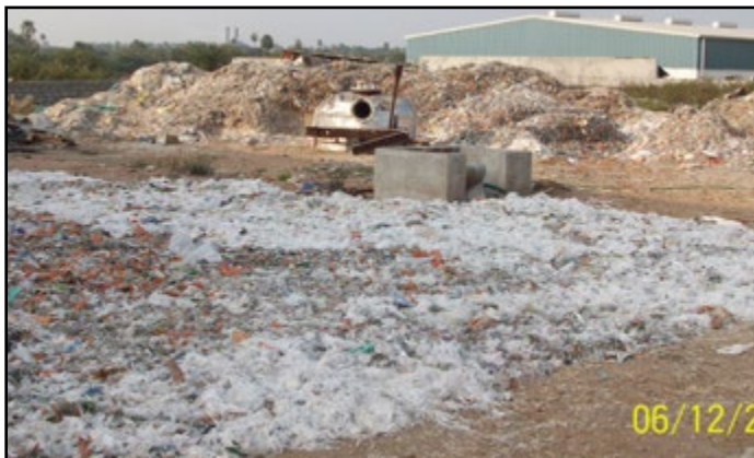
Mixed Plastics Waste being dried before feeding into the reactor
