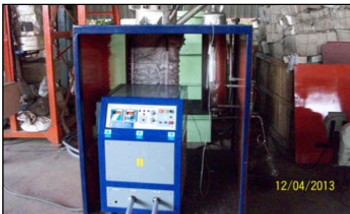
Small Size Pyrolysis Plant - 50 Kg Batch
